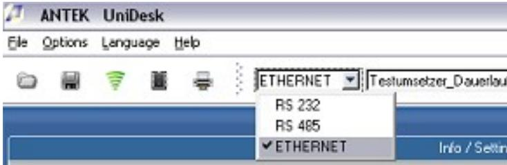
If a RS485 junction is active, during the first junction setup each device found on the RS485 BUS will be entered into the list element of the toolbox. With the DropDown element each device that is active on the BUS can be selected. If further devices are subsequently added to the BUS, the BUS must be re-read-in. This can be carried out by actuating the button "Disconnect" in the toolbox and then by re-activating the "Connect".
