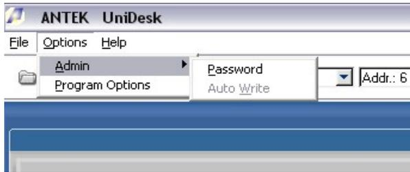
Some parameters can be protected by a password. Only after having entered the correct password via this menu item, the parameters become visible and can then be edited. When entering any false password (or by a dummy input) the protected parameters are hidden automatically.
