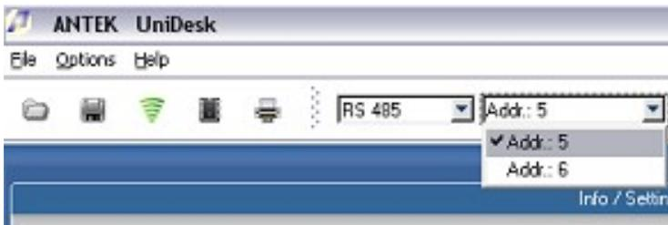
ANTEK - devices that are connected over a network are also activated by using the drop-down box to connect. Each device name has its own IP address deposited (see 5.3.8.3 Ethernet).
